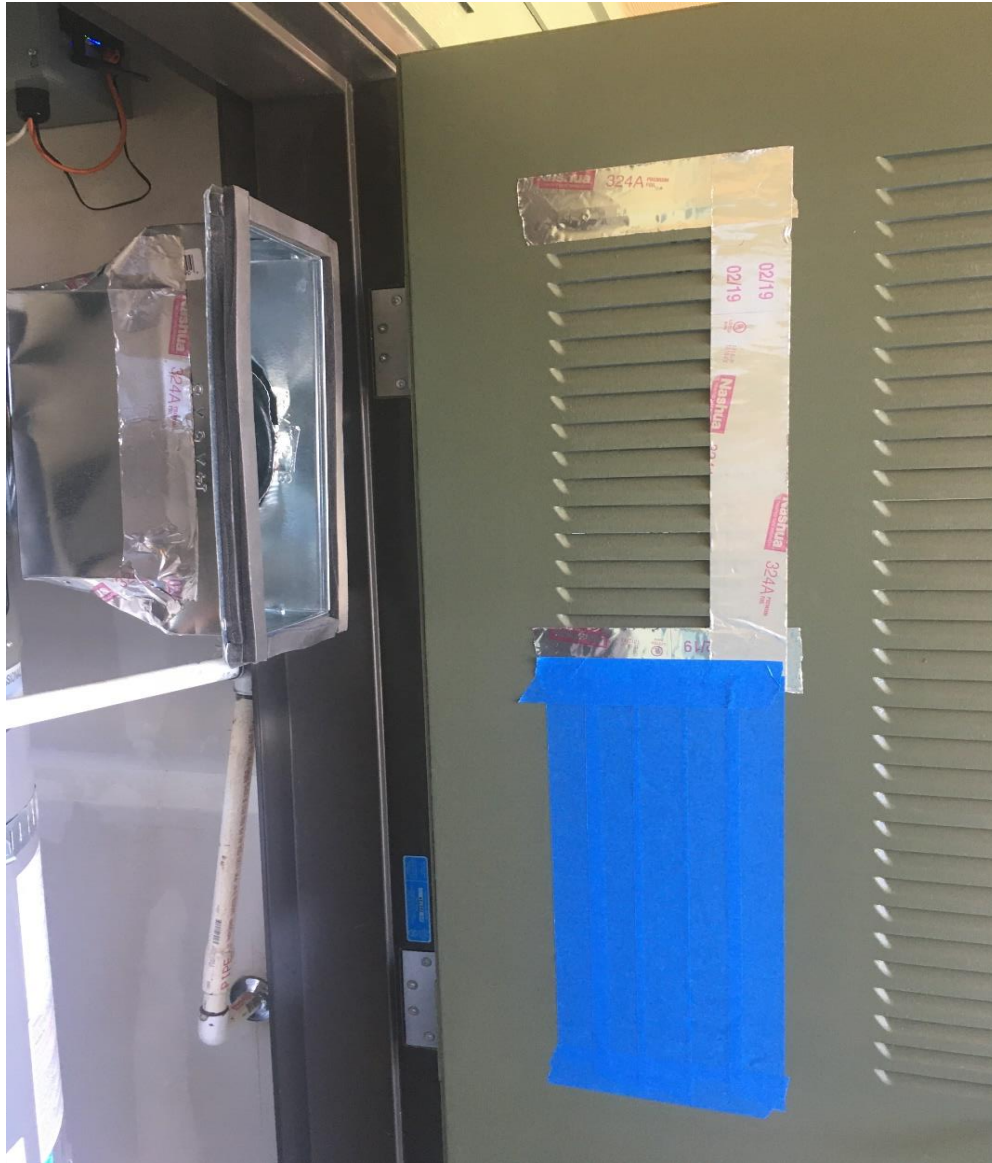
Figure 3: Louvered Door Interior Panel Taped to Prevent Exhaust Air Backflow
